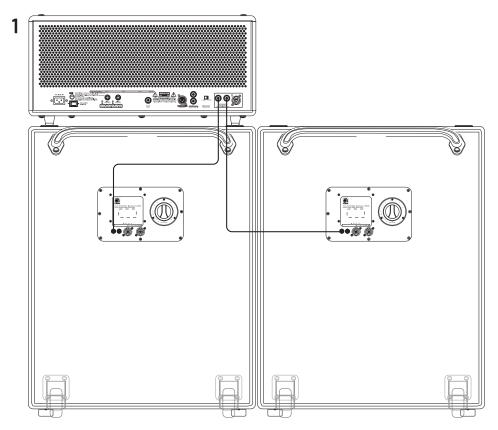
In example 1 above, a speaker cable with 1/4" ends connects from one speaker output of the amplifier to the speaker input of the Ampeg SVT-410HLF cabinet. An additional cabinet may be connected by attaching another speaker cable from the remaining 1/4" speaker output of the next of cabinet.
