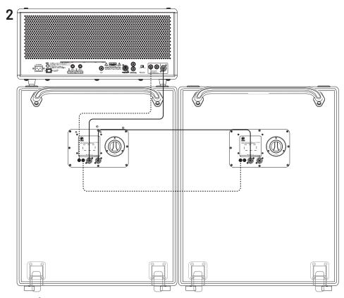
Example 2 above is not as common, but is great for daisy-chaining multiple cabinets. You may connect a speaker cable with 1/4" or Speakon ends from one speaker output of the amplifier to the speaker input of the Ampeg SVT-410HLF cabinet. An additional cabinet may be connected by attaching another speaker cable from an open jack (thru) to the input jack of the next cabinet. Multiple cabinets may be daisy-chained this way.
